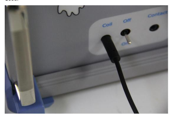
2. The connection between the adapter and the coil must also be tight. Even a small gap will interfere with the normal function of the coil.
