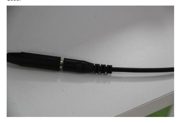
Here is the full view showing the correct connection among the socket, adapter and the coil.
